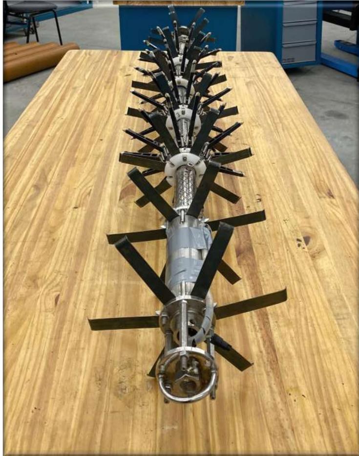
Figura 2.4: PIG palito multidimensional.
